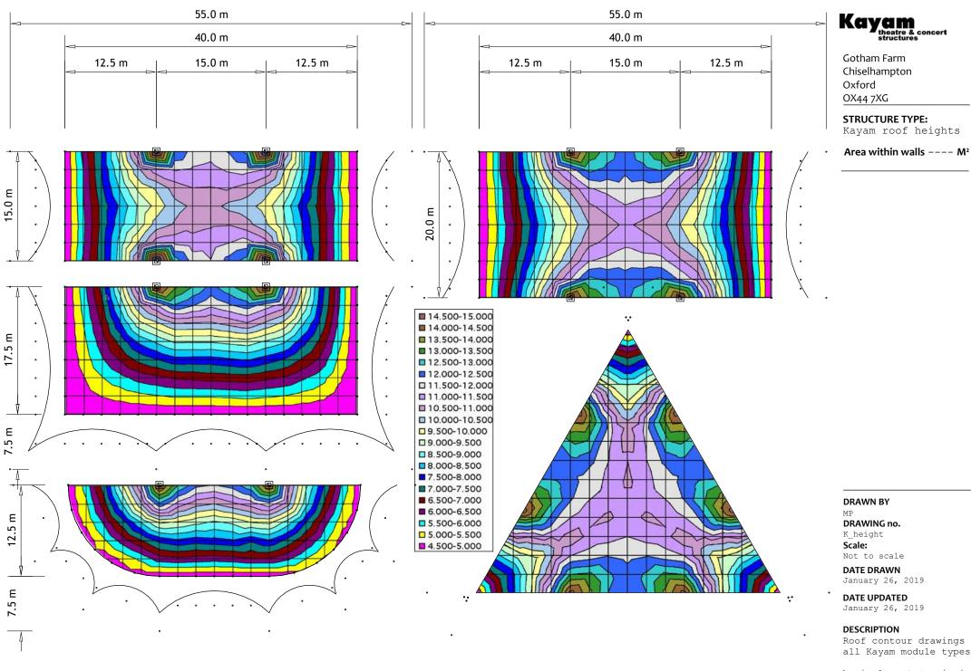
Roof contour drawings for all Kayam module types.
